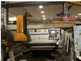
Bridge saw Breton Easycut FE800 Year 2006 3 axis Motorized rotating table. Tilting table. Variable disc speed by inverter Max disc 800 mm Min disc 400 mm Manual disc tilt 0 - 90 degrees
